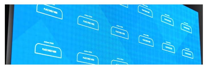
**PROTECTION** A protective film on the face of the LED is used to provide durability for the panels. Made of a sealing spray, the protective film encases the LEDs without affecting the refracting index, light transmission or brightness loss. The film also adds anti-collision, anti-shock, anti-UV, water proofing, dust resistance, and heat dissipation that extends the life span.
